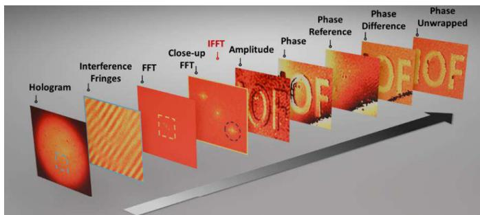
**Fig. 1** Image reconstruction process, a sequence of steps used in Fourier off-axis holography are implemented together with the undetected photons scheme to reconstruct phase and amplitude information.
