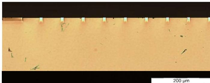
Figure 1. Microscope image of the crystal input facet with 20X magnification. Each waveguide input channel has width ranges from 3-7  $\mu\text{m}$ .
