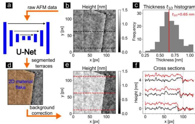
Figure 1. Schematics of AFM image analysis using a U-Net.
