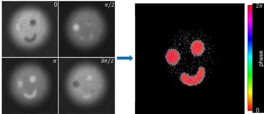
Figure 1. Intensity distributions of four different interferograms, each carrying a given phase shift. After processing, the interferograms are transformed into the object's phase distribution.
