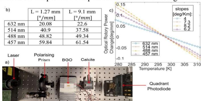
Figure 2. a) Experimental setup. b) Table of optical rotatory powers measured on room temperature. c) Optical rotatory power change with temperature
