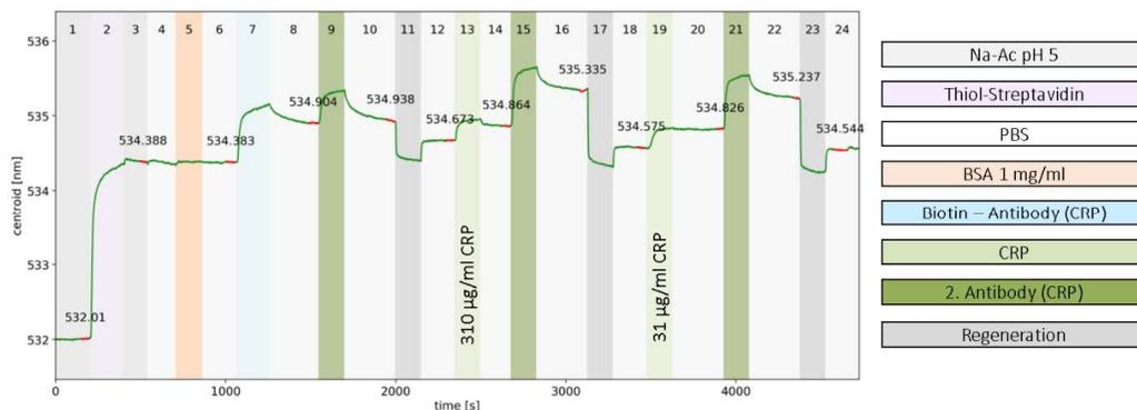
Figure 1. Sensogram (LSPR peak wavelength centroid plotted over time) of the various steps (including sensor functionalization and control experiments) of a CRP protein detection assay. Different colors mean different (buffer/analyte) solutions. (From [3])
