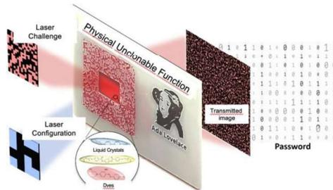
Figure 1. Scheme of the PUF token and its internal configuration (blue pattern), challenge interrogation (red pattern), transmitted speckle pattern, and generated password.
