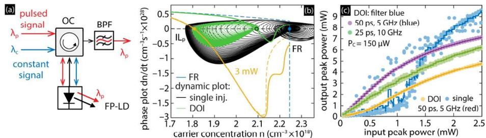
Figure 1. (a) NLE operating principle. (b) FP-LD phase plot under single injection and DOI. (c) NLE output power variation for different repetition rate, pulse width and BPF central frequency.
