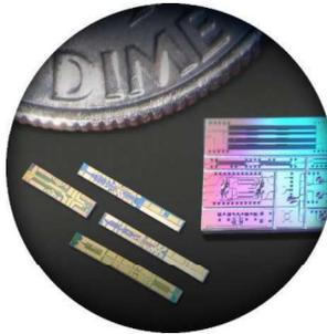
Figure 1. Various photonic integrated circuits in Indium Phosphide and Silicon.
